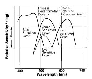
\* Sensitivity equals the reciprocal of the exposure (ergs/cm²) required to produce a specified density.
